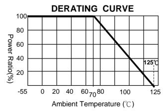
Power rating or current rating is in the case based on continuous full-load at ambient temperature of  $70^{\circ}$ C. For operation at ambient temperature in excess of  $70^{\circ}$ C, the load should be derated in accordance with figure of derating Curve.
